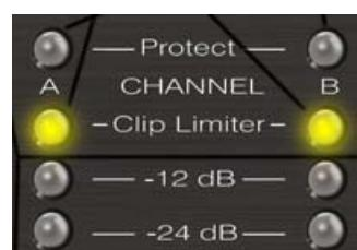
**i** Make sure this LED is not alight permanently ! No extra power is obtained in this way losing dynamics and sound quality.
